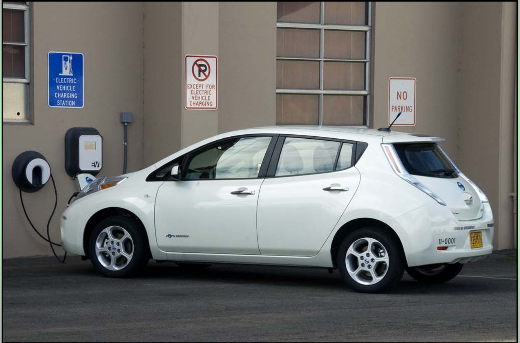
EVSE Level 2 – ODOT Workplace Charging
